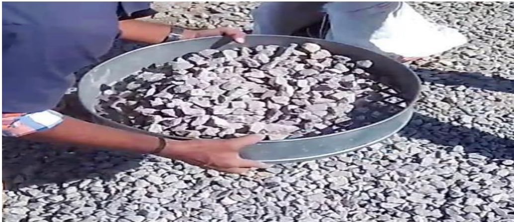
Figure 2.3 By using IS Sieve 20mm the Coarse aggregate is sieving by hand
