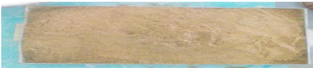
Figure 2.2 Fine aggregate (Sand)
